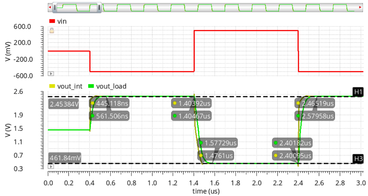
Figure 6. The transient response when the input is 1V. The settling time for both rising edge and falling edge can be derived in this plot.
